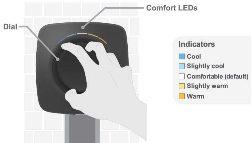
Figure 2: Beanbag thermostat 500 series user interface
